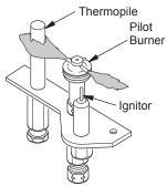
Figure 42 - Correct Pilot Flame Pattern
